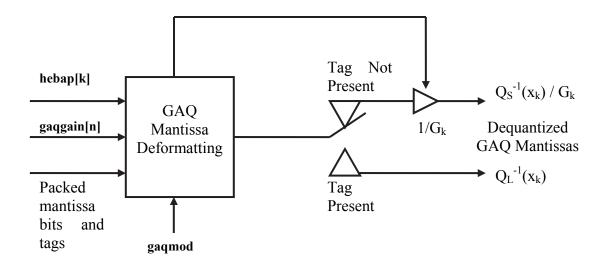
Figure E3.1 Flow diagram for GAQ mantissa dequantization.
