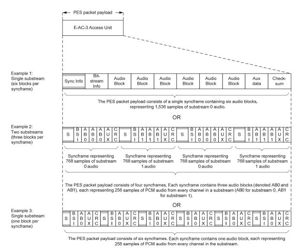
**Figure G.1** E-AC-3 **sync**frames within the PES packet payload.
