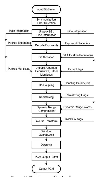
**Figure 6.1** Flow diagram of the decoding process.
