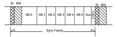
**Figure 5.1** AC-3 synchronization frame.
