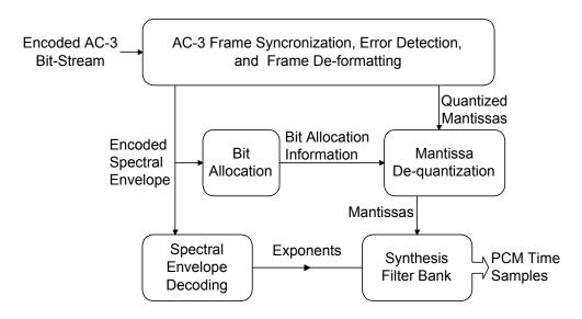
Figure 2.3 The AC-3 decoder.
