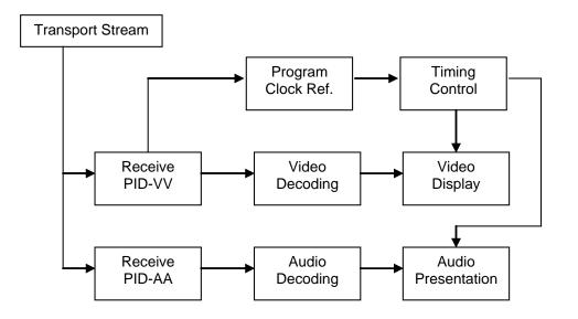
Figure D9 Acquisition of audiovisual components.
