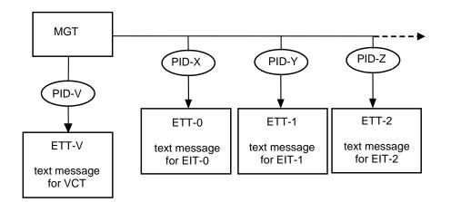
Figure 5.2 Extended Text Tables (ETTs) defined to carry text messages for describing virtual channels and events.
