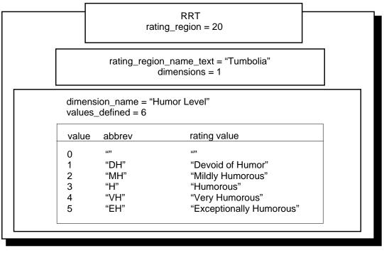
Figure D6 An Instance of a Rating Region Table (RRT).
