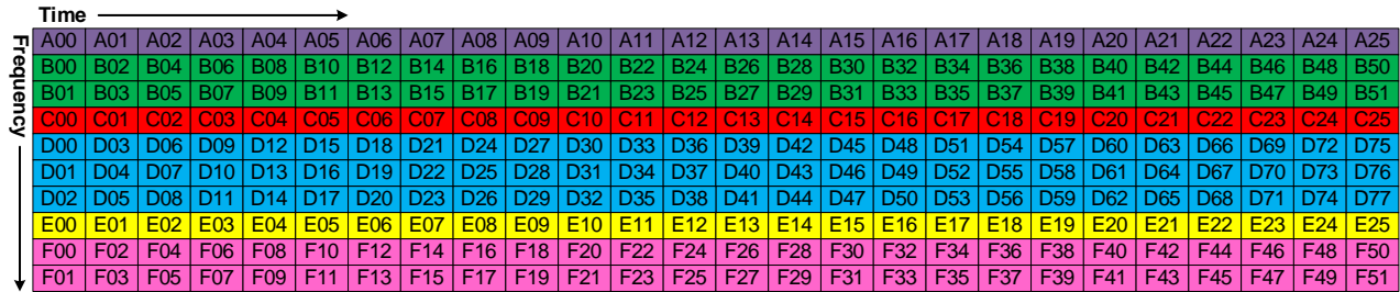
Figure 7.24 Example of frequency division multiplexing of PLPs.
